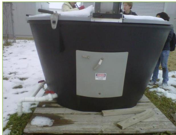
*Pictured: the Earth Tub as it is currently installed at Carleton College in Northfield, MN. A standard shipping flat serves as the Earth Tub's base. Electricity is brought in from above. Drainage pipes funnel liquid to in-ground 5-gallon pail.*
